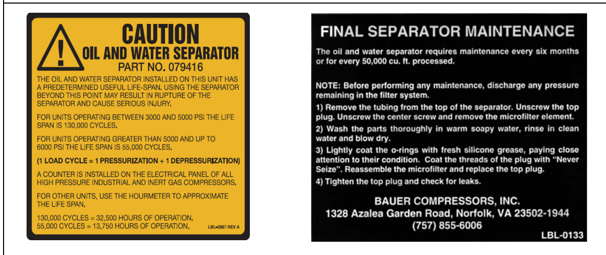
Figure 4-3 Oil and Water Separator Labels
